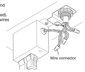
5 Replace the wire cover with the screws removed previously. Make sure that all wires are connected properly and enclosed inside of the wiring compartment.
