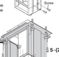
7 Set 4 flange-nut (not supplied) on the threaded rods as shown for fixing the supplied hanging brackets later.
