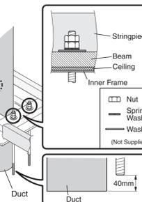
5 (1) Pull out the inner frame after removing 4 screws fastening to the outer frame.
