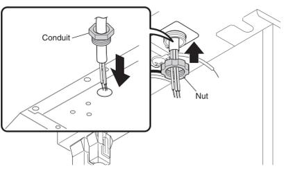
4 Connect wires tightly and securely using wire connectors (not supplied). Connect the electrical wires as follows:
