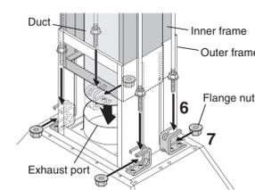
7 Fix the range hood unit by adding 4 flange nuts (not supplied) to the threaded rods as shown.
