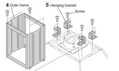
6 With inserting the inner frame into the outer frame and the exhaust port into the duct, lift up the range hood unit and pass the threaded rods through the hanging brackets as shown.
