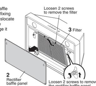
3 Detach the filters by turning the fixing knobs counter-clockwise, and disengaging them from the supporting groove.
