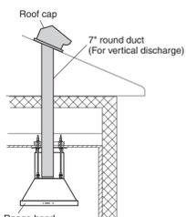
**CAUTION:** Install the range hood unit using anchor bolts durable enough to support its weight (withstand load: more than 441lbs. (200kg/pc). Otherwise, it may be detached and fall down.
