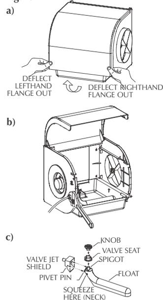
CLEANING OR REPLACING THE WATER PAN
