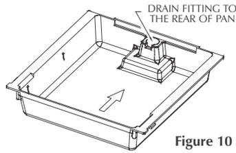
**IMPORTANT NOTE: IF YOU ARE PLANNING ON INSTALLING A DRAIN TUBE (NOT SUPPLIED) DRILL OUT THE DRAIN FITTING AS SHOWN IN THE SECTION "OVERFLOW DRAIN CONNECTION" BEFORE INSTALLING THE DRUM. ONLY DRILL OUT THE DRAIN FITTING IF YOU ARE INSTALLING A DRAIN TUBE. YOU WILL HAVE PURCHASE THE TUBE SEPARATELY.**
