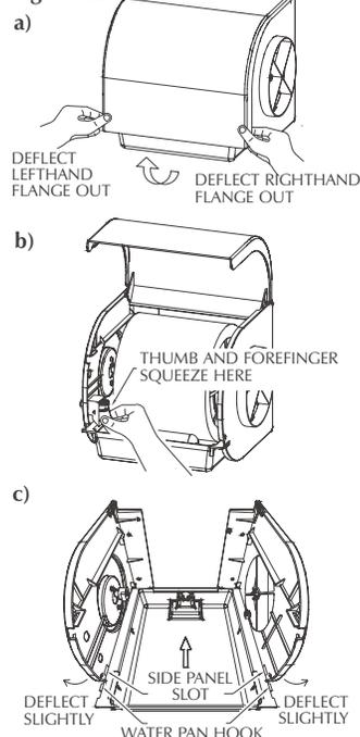
neck of the float squeeze firmly and this will disengage the 2 pivot pins from the holes at the sides of the valve jet shield. (Fig. 42b)
