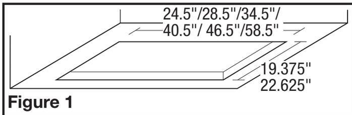
**NOTE:** The hood must be mounted a minimum of 24" and a maximum of 36" from the cooking surface.
