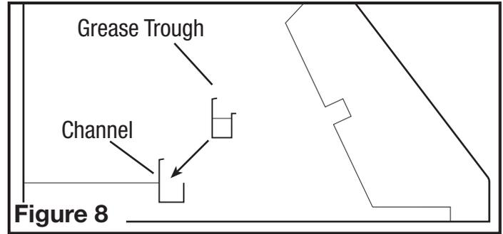
3. Install the baffle filters and any spacers included with the unit by inserting the top of the filter into the top channel of the hood, then slide the bottom of the filter into the bottom channel. The filters have a top and a bottom. The bottom of the filter will have small drain holes. These holes must be facing down towards the grease trough to be effective (Figure 9).
