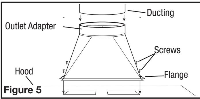
3. When there is access to the top of the unit, connect the ducting to the duct collar and secure in place using tape to seal all joints (Figure 5).
