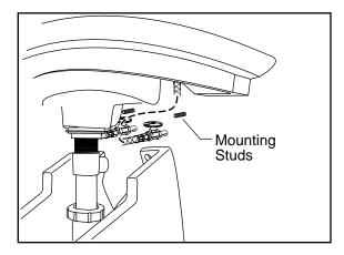
Connect water supplies lines and drain pipe connections. Turn water on and check for leaks.
