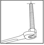
ANCHOR SCREW INSTALLATION Install lavatory anchor screws leaving 1-5/8" threaded end exposed as illustrated. Position semi-pedestal under bottom lip of sink. While holding semi-pedestal in position reach through the access area between the lavatory and semi-pedestal and mark the location of anchor holes. Remove semi-pedestal and predrill 3/16" (4-5mm) dia. holes at locations marked. Install 1/4" x 3" lg studs leaving 1-1/4" exposed. Use same anchor screw installation as in 2a.
