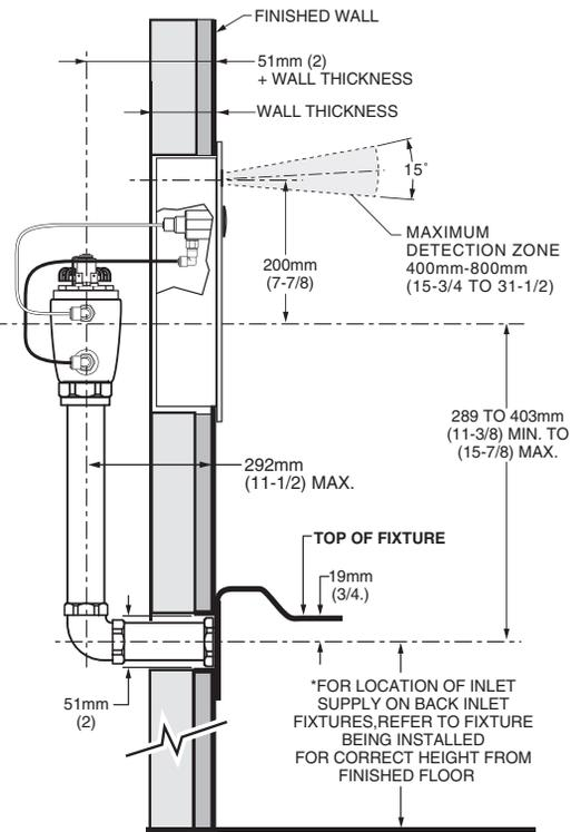
\*Note: The Critical Line (-C-L-) on Vacuum Breaker must typically be 6" (152mm) min. above fixture. Consult Codes for details.
