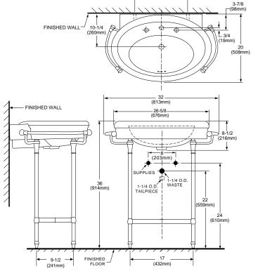
DIMENSIONS SHOWN FOR LOCATION OF SUPPLIES AND "P" TRAP ARE SUGGESTED. ANCHOR SCREWS FOR LAVATORY AND PEDESTAL NOT INCLUDED. FITTINGS NOT INCLUDED AND MUST BE ORDERED SEPARATELY.
