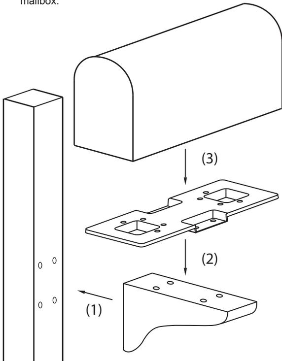
For double configurations (one mailbox on each side of the post), assemble both support arms (5512) as shown above. Double configurations can be used for Coronado, Bellevue or Oasis Jr. Mailboxes.
