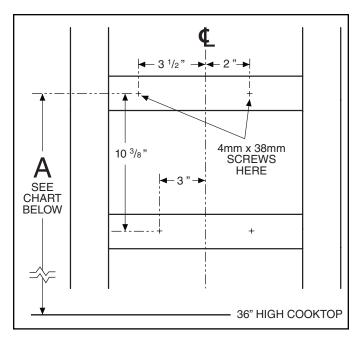
Construct wood wall framing that is flush with interior surface of wall studs. Make sure the framing is centered over installation location.
