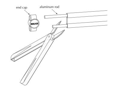
Caution - For shortening the track, use a Track Cutting Shear (230990). Cut the track carefully to avoid damage to the conductive braiding.
