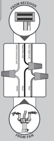
Using an orange wire connector from the Thardware bag, connect the black wire (ungrounded) from the ceiling to the black wire from the receiver (marked "live in"). Connect the white wire (grounded) from the ceiling to the white wire from the receiver (marked "neutral in" or "common in").
