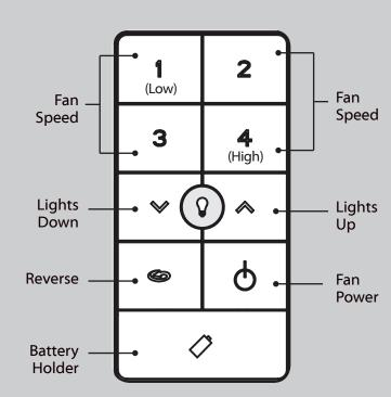
Quickly press the up or down arrow to turn the lights off and on. Hold the up or down arrow to raise or dim the light level. The reverse button changes the direction that the blades turn. The power button turns the fan off and on.
