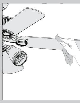
For cleaning the fan, use soft brushes or cloths to prevent scratching. Cleaning products may damage the finishes.
