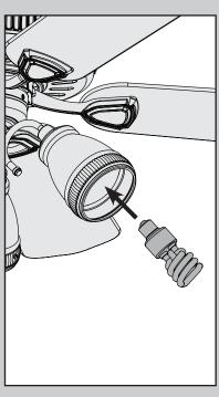
Install the CFL bulbs into the sockets. When necessary, replace with bulbs of same wattage.
