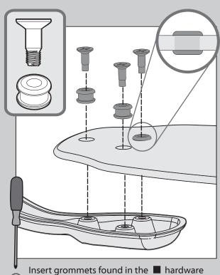
bag into the holes in the hardward bag into the holes in the blades, then secure each blade to a blade iron with screws found in the hardware bag.
