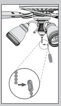
Connect the pull chain pendant to the short chain coming from the switch housing.
