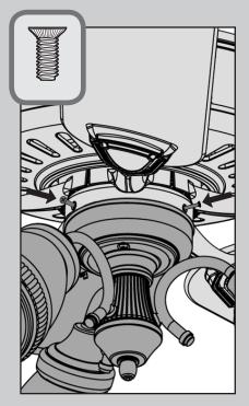
Install the three switch housing screws, found in the ≡ hardware bag.
