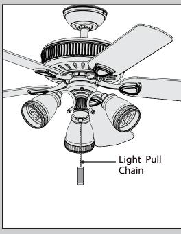
The light pull chain controls the power to the light fixture: on and off.
