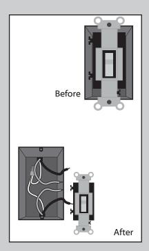
After removing the switch plate cover, remove all wiring from the switch.
