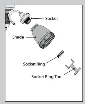
Remove the socket rings from the sockets.
