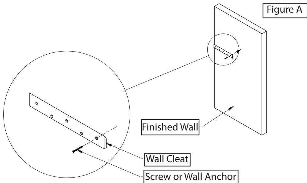
NOTE: Due to vast difference in building materials, wall anchors and screws are not provided but are recommended throughout instructions.
