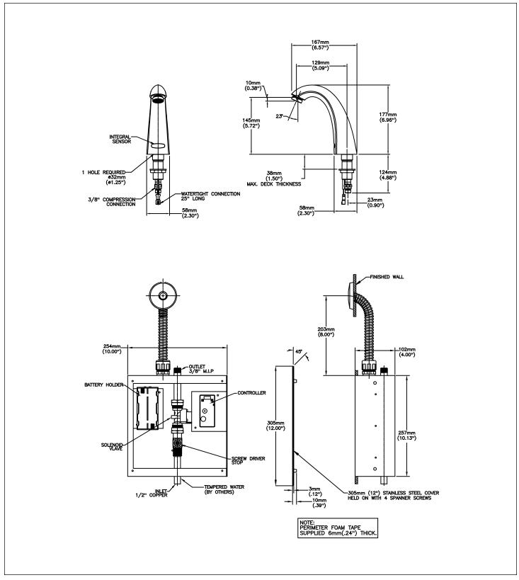
Delta reserves the right (1) to make changes to specifications and materials, and (2) to change or discontinue models, both without notice or obligation. Dimensions are for reference. Measurement may vary plus or minus 6mm(0.25"). Mounting locations are suggested only. Check with local codes for requirements in your area. This spec was produced March 08, 2012.
