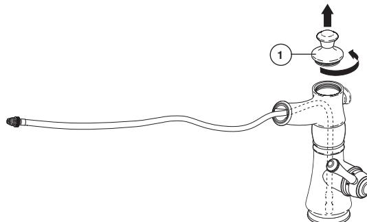
**Hose Assembly Removal and Replacement Instructions** - Note: Color and size of hose will differ from production assembled model. This RP hose is slightly smaller in diameter with shorter end fittings to help you install. Your flow rate will not be affected.
