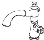
When removing and replacing the hose assembly for this model, it is necessary to remove the top cap (1), as shown, to help guide the hose down into the hub.
