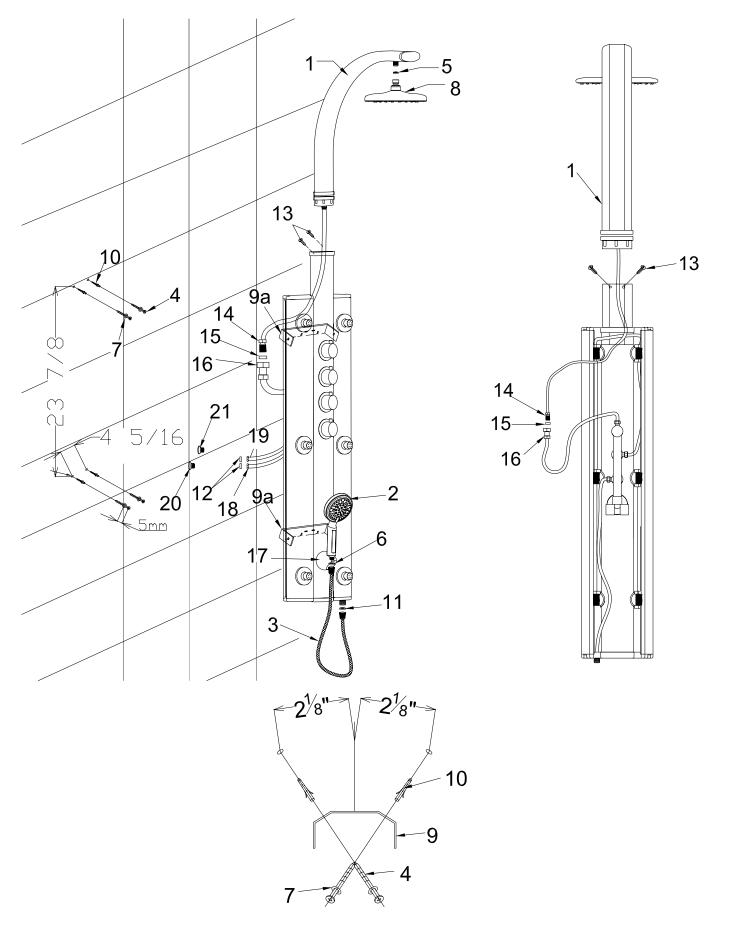
Refer to the technical diagram to choose the proper location for your shower column. You can adjust the column's vertical position based on the person's height. Measurements given in the technical diagram are based on the average human height ( $68^{\circ} - 70^{\circ}$ ).
