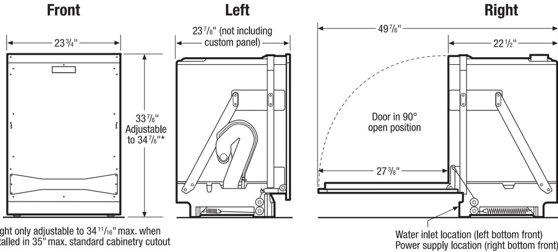
\*Height only adjustable to 34 11/16" max. when installed in 35" max. standard cabinetry cutout
