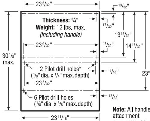
\*Optional holes for adding 1/2"- #7 screws which slip into rectangular openings of metal panel to help locate custom door panel for other outside screw attachment
