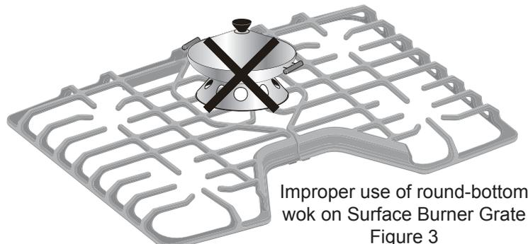
Improper use of round-bottom wok on Surface Burner Grate
