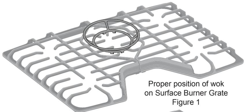
Proper position of wok on Surface Burner Grate
