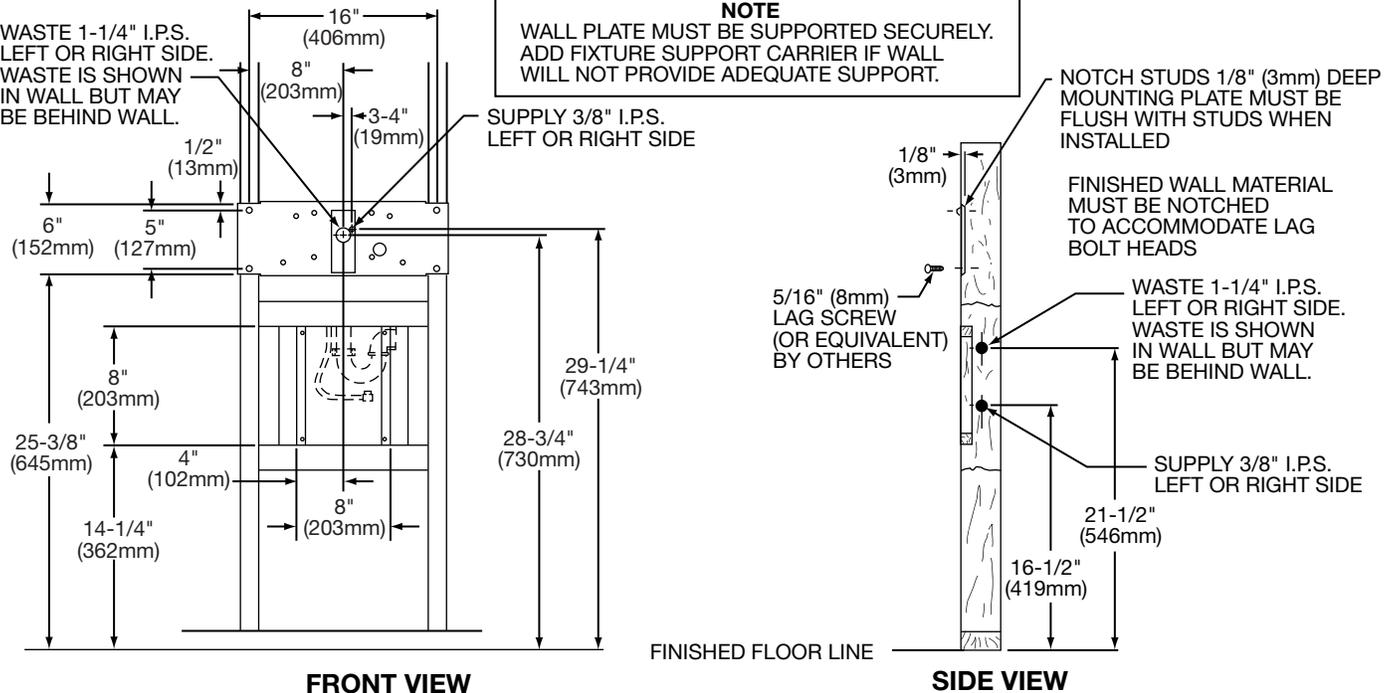
NOTCH STUDS 1/8" (3mm) DEEP MOUNTING PLATE MUST BE FLUSH WITH STUDS WHEN INSTALLED
