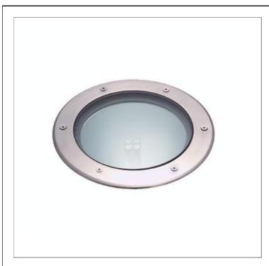
Circular CFL up-light. 120V input, integral ballast. Tempered safety glass lens. Symmetrical diffuser of anodized aluminum. Stainless steel outer trim. Cast aluminum metal body with powder coat finish. PVC mounting housing included.
