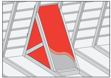
Frame out the shaft, line with plasterboard, and ensure that the shaft is clad with roofing insulation in the roof cavity. This will reduce heat transmission from the roof cavity into the home in summer, and help reduce heat loss from the home in winter.
