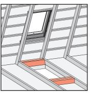
Prepare the hole in the ceiling using trimmer timbers in the same way trimmers are used in roof and wall construction.
