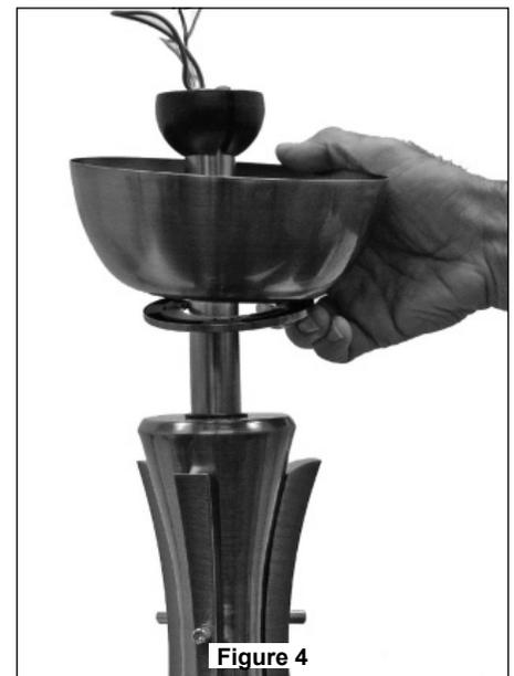
4. Re-assemble the Canopy Screw Cover, Canopy, and downrod hanger ball assembly. Reinstall the Hanger Ball (Figure 4) on the Downrod as follows. Position the Pin through the two holes in the Downrod and align the Hanger Ball so the Pin is captured in the groove in the top of the Hanger Ball. Pull the Hanger Ball up tight against the pin. Securely tighten the setscrew in the Hanger Ball. A loose setscrew could create fan wobble.
