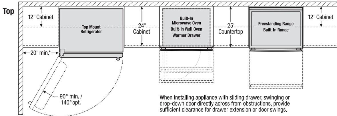
When installing appliance with sliding drawer, swinging or drop-down door directly across from obstructions, provide sufficient clearance for drawer extension or door swings.
