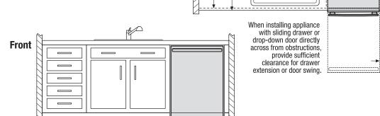
When installing appliance with sliding drawer or drop-down door adjacent to wall. cabinet, or other obstruction that extends beyond front edge of appliance, allow 2" minimum clearance between drawer or door and obstruction.
