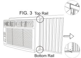
Your air conditioner is designed to install in standard double hung windows with opening widths of 23 to 36 inches (584 mm to 914 mm) (FIG. 4A, FIG. 4B).
