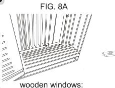
Place the frame lock between the frame extensions and the window sill as shown (FIG. 8A for wooden windows), (FIG. 8B for Vinyl-Clad windows).
