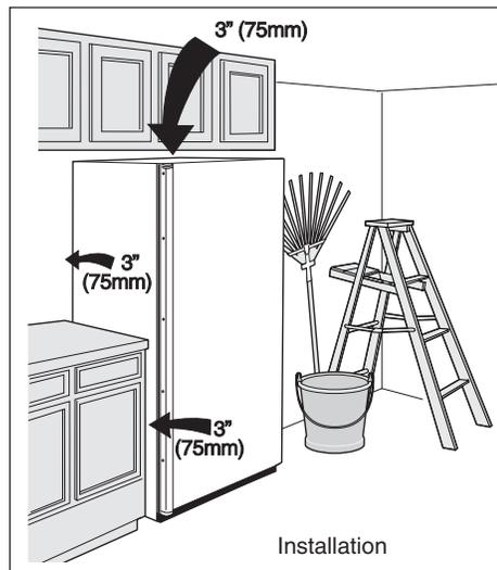
**NOTE:** The exterior walls of the refrigerator may become quite warm as the compressor works to transfer heat from the inside. Temperatures as much as 30° F warmer than room temperature can be expected. For this reason it is particularly important in hotter climates to allow enough space for air circulation around your refrigerator.
