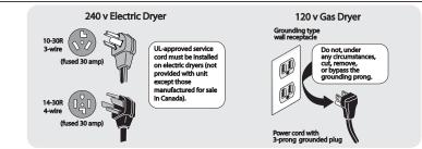
Avoid fire hazard or electrical shock. Do not use an adaptor plug or extension cord or remove grounding prong from electrical power cord. Failure to follow this warning can cause serious injury, fire or death.
