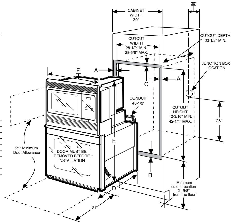
**MOST 30" WALL CABINETS CAN BE USED WITH THIS UNIT. THE OPENING BETWEEN THE INSIDE WALLS MUST BE AT LEAST 28-1/2" WIDE.**
