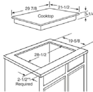
\*Depth of unit at conduit connection location (rear) is 6-1/4" on models PP975/945 and 4-3/16" on models CP350/650, PP944/962/932/912, and JP656/356/336. Depth of unit at baffle (front) is 4-5/8" on models PHP960/900.
