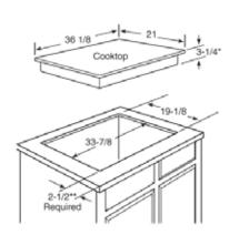
\*Depth of unit at conduit connection location (rear is 6-1/4" on models PP975/945 and 4-3/16" on
