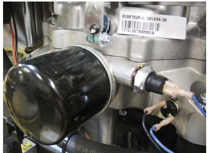
Figure 3.4 – Low Oil Pressure and High Temperature Switches
