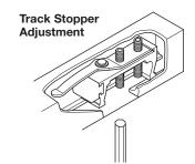
The retaining force can be adjusted with a hex key.
