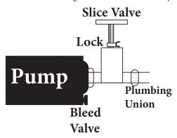
**The Spa Pump** pushes water through the plumbing lines into the jets. Pumps are turned on and off by pressing the button(s) on the topside controls. The number and speed of the pump varies by spa model.
