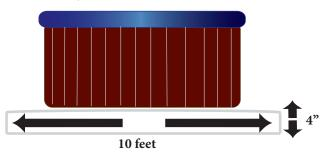
To allow for adequate drainage away from the spa, Concrete should slope 1/2" over 10' from the center.
