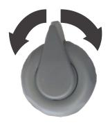
The Diverter Valve is a large rotating dial on the topside of the spa used to control flow of the water between sections of the spa controlled by each pump in the spa. The diverter valve rotates right and left. Do not over turn the diverter valve which has built in "stops". Forcing the valve to turn past it's built in "stop" will damage the spa.
