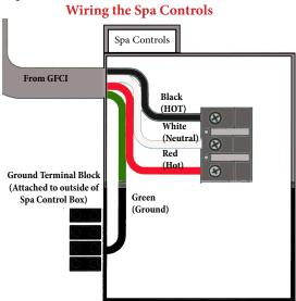
A green colored terminal is provided in the control box. To reduce the risk of electrical shock, connect this terminal or connector to the grounding terminal of your electrical service or supply panel with a continuous green insulated copper wire.
