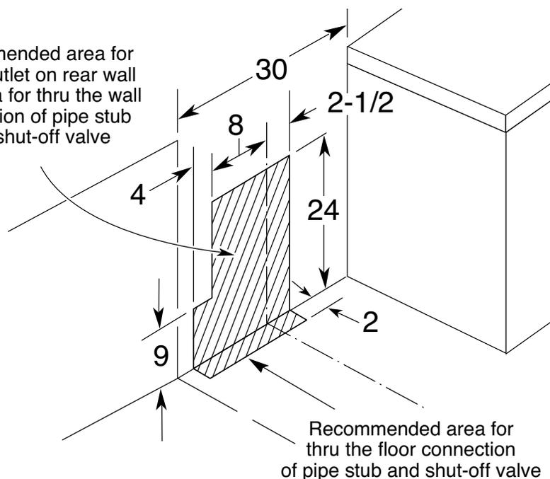
Recommended area for thru the floor connection of pipe stub and shut-off valve
