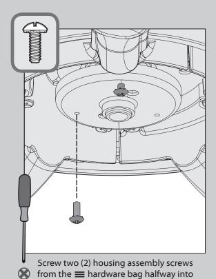
the motor housing. It does not matter
