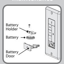
Before operating the wall control, press the battery door to eject it. Using a Phillips head screwdriver, remove the battery holder. Install the battery with the positive (+) side facing downward. Secure the battery by reinstalling the battery holder. Finally, reinstall the battery door into the wall control. When necessary, replace with CR2032 battery.
