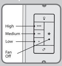
The Fan Off button only turns the fan off. To turn the fan on, press one of the fan speed buttons. They are located next to the Fan Off button.
