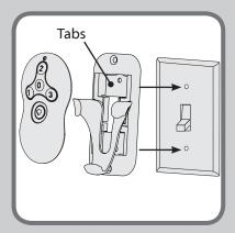
To install the transmitter cradle, remove the two screws holding your switch cover plate. Do not remove the cover plate. Orient the cradle by lining up the two mounting holes with those on the cover plate. Insert and tighten the screws. Do not over tighten. Note: For paddle-style switches, break off the tabs on the cradle by pushing outward.
