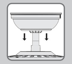
Remove the canopy. If uncertain how to remove it, reference the fan's owner's manual. With wiring exposed, it may be helpful to note existing wire connections or take a digital photo for reference. Remove the wire connectors that connect the wires from the outlet box to the fan, leaving the grounding wires connected.
