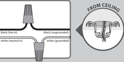
CONNECT WIRES FROM RECEIVER TO WIRES FROM OUTLET BOX - Using an orange wire connector connect the black wire (ungrounded) from the ceiling to the black wire from the receiver (marked "live in"). Connect the white wire (grounded) from the ceiling to the white wire from the receiver (marked "neutral in").
