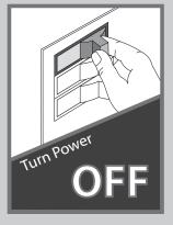
Before installing the Universal Remote Control Receiver, use the pull chains to set the fan speed to HIGH and the light to ON. Be sure power is OFF before proceeding with installation.
