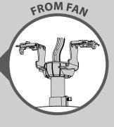
CONNECT WIRES FROM RECEIVER TO FAN - Using the blue wire connectors connect the white wire from the receiver (marked "common out") to the white wire from fan. Connect the black wire from the receiver (marked "fan out") to the black wire from the fan. Connect the blue wire from the receiver (marked "light out") to the blue wire (or possibly black with white stripe) from the fan.
