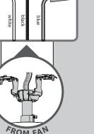
Using an orange wire connector from the ★ hardware bag, connect the black wire (ungrounded) from the ceiling to the black wire from the receiver (marked "live in"). Connect the white wire (grounded) from the ceiling to the white wire from the receiver (marked "neutral in" or "common in").
