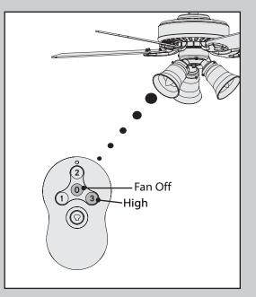
Note: The remote must be paired before the fan will operate. Within 3 minutes of restoring power to the fan, press both the Fan Off button and the High button for at least 4 seconds. Your fan will turn on low to indicate successful syncing. If it does not, turn off power to your fan, wait 1 minute then try again. If using the transmitter with multiple fans, repeat this process for each fan.
