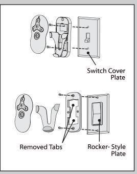
To install the transmitter cradle, remove the two screws holding the switch cover plate. Do not remove the cover plate. Orient the cradle by lining up the two mounting holes with those on the cover plate. Insert and tighten the screws. Do not over tighten.
