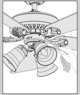
For cleaning the fan, use soft brushes or cloths to prevent scratching. Cleaning products may damage the finishes.
