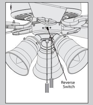
To switch the direction of air flow, move the reverse switch to the opposite position.
