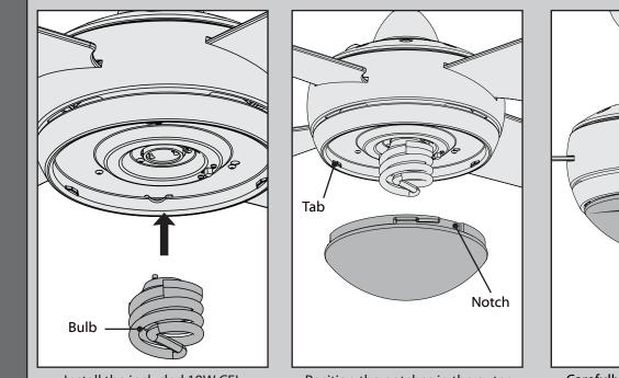
Install the included 18W CFL bulb. When necessary, replace with bulbs of same wattage. Position the notches in the outer rim of the globe so they line up with the tabs on the light kit ring. Carefully lift the globe up inside the light fixture as far as it will go. Rotate the globe in a clockwise direction until it is held tightly in place by the three tabs.
