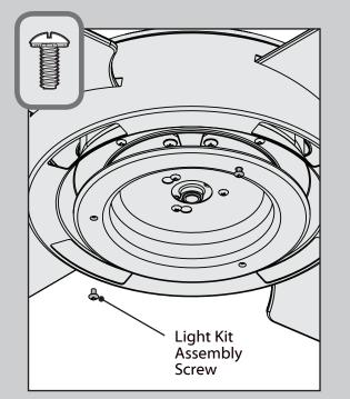
Partially install two of the light kit assembly screws, found in the  $\equiv$  hardware bag.
