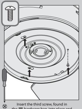
the ≡ hardware bag, into place and then tighten all three screws.
