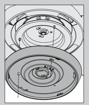
Align the keyholes in the light kit ring with the partially installed screws. Lift the light kit ring in place and rotate counterclockwise to situate the screws in the narrow ends of the keyholes.
