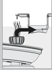
DO NOT PICK THE FAN UP BY THE CANOPY OR WIRES. Place the downrod ball into the slot in the ceiling bracket.
