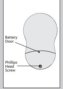
To access the battery compartment, remove the small Phillips head screw that secures the battery door to the transmitter assembly. The battery should be installed with the positive (+) side up. Replace with a CR2032 battery when necessary.
