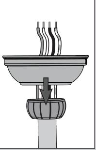
Put the wires and downrod through the canopy. Let the canopy sit loosely on top of the fan.
