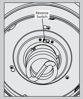
To switch the direction of air flow, move the reverse switch to the opposite position. You will need to remove the light kit glass to do so.
