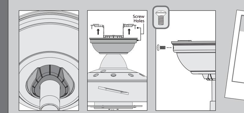
Position the canopy so that, when lifted into place, the canopy fits into the hanging bracket as shown. Lift the canopy into place so that the screw holes are aligned.
