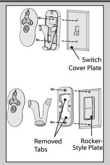
To install the transmitter cradle, remove the two screws holding the switch cover plate. Do not remove the cover plate. Orient the cradle by lining up the two mounting holes with those on the cover plate. Insert and tighten the screws. Do not over tighten. **Note:** For rocker-style cover plates, break off the tabs by pushing outward.
