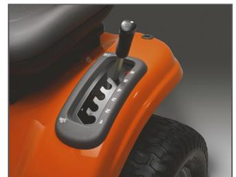
**FENDER-MOUNTED CUTTING HEIGHT ADJUSTMENT**
