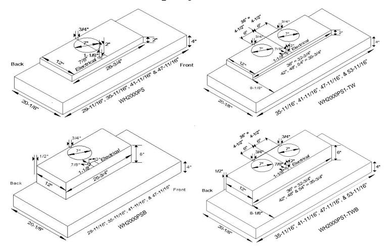
CEILING HEIGHT = \_\_\_\_\_ COUNTER HEIGHT = 36" MOUNTING HEIGHT = 36" HOOD HEIGHT = 6"
