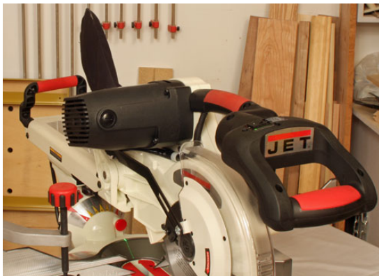
The handles are placed for maximum control and comfort in operation and when carrying the saw to the job.
