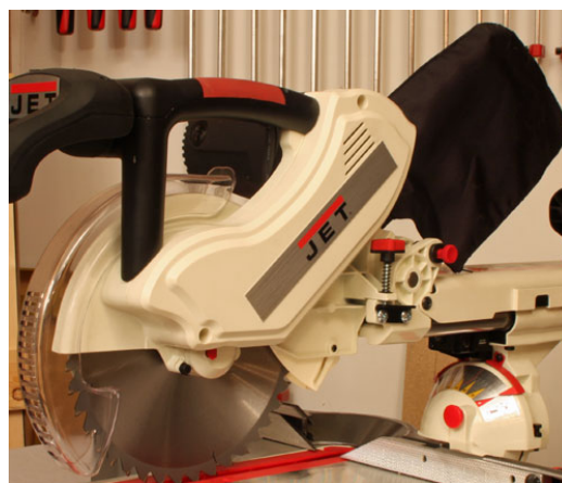
The blade shroud and dust bag help keep the work area clear.
