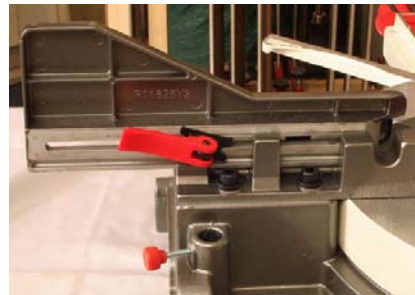
The spacious work table (left) provides lots of support for all project types. Note the swing-out support arms. The vertical fence extensions (right) are tool-free thanks to this cam lock on the rear.
