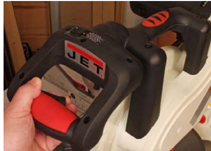
The operating arm is spring assisted (left) and has its controls placed for easy access and use. The operating handle (right) features a built-in On/Off trigger and a separate switch for the laser so it can be used only when desired.
