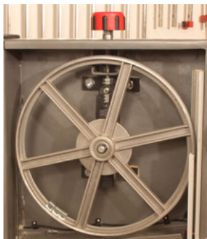
The blade wheels (left) are balanced and mounted on ball bearings for smooth running. We included easy blade tensioning (right) as well as a single lever for relaxing blade tension when not in use.
