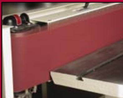
The JET® Oscillating Edge Sander showcases a unique oscillating feature. Oscillation of the belt means the sandpaper never runs a true straight line, which allows the unit to sand with more of the usable sandpaper and eliminates sanding lines. With a large sanding surface, you can process both the edge and surface of many different board sizes. Contour sanding is also an option when using the large built-in table around the drum over the motor.
