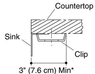
\*Allow clearance around the back sink rim for clip attachment.
