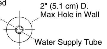
For slip-fit spout, 5/8" OD tube must extend 4-3/4" (12.1 cm) beyond finished wall.
