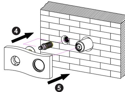
Place sufficient Teflon tape on connecting pole 15. Screw it into corresponding screwed hole of valve 17 (If the connecting pole is too long please shorten it with a saw; refer to dimensions for detail size). Install decorative board 13 and Fixing board 14 to valve.
