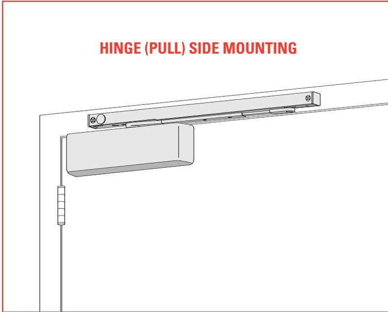
*The 4040SE SENTRONIC® is a heavy duty, non-handed, non-sized closer/holder designed to provide single point hold-open for fire and smoke barrier doors. The door is held open until current interruption releases the holding mechanism and the door closes. Single lever (track) arm closer is specifically designed for interior doors. Choice of finishes, track functions, and installation accessories meet virtually all life safety requirements.*
