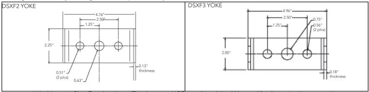
Yoke Mounting Plate Template Note: This drawing is NOT to scale and should be used for dimensional purpose only.
