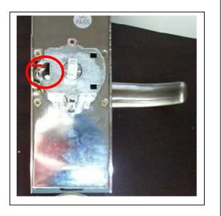
When the front mount is in place, hold the back mount rubber gasket against the back side of the door and place the back mount over the gasket and onto the stem protruding from the front mount.
