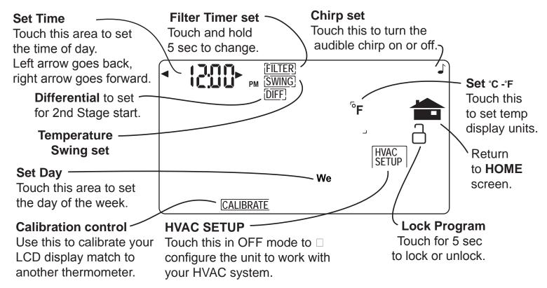
PROGRAM Screen The stand alone PROGRAM screen sets the ÆÛË € control for your home HVAC system with out a central controller. Press and hold PROG for 10 sec to access it. After that it is displayed when you press the PROG button. [See page 8 for details]
